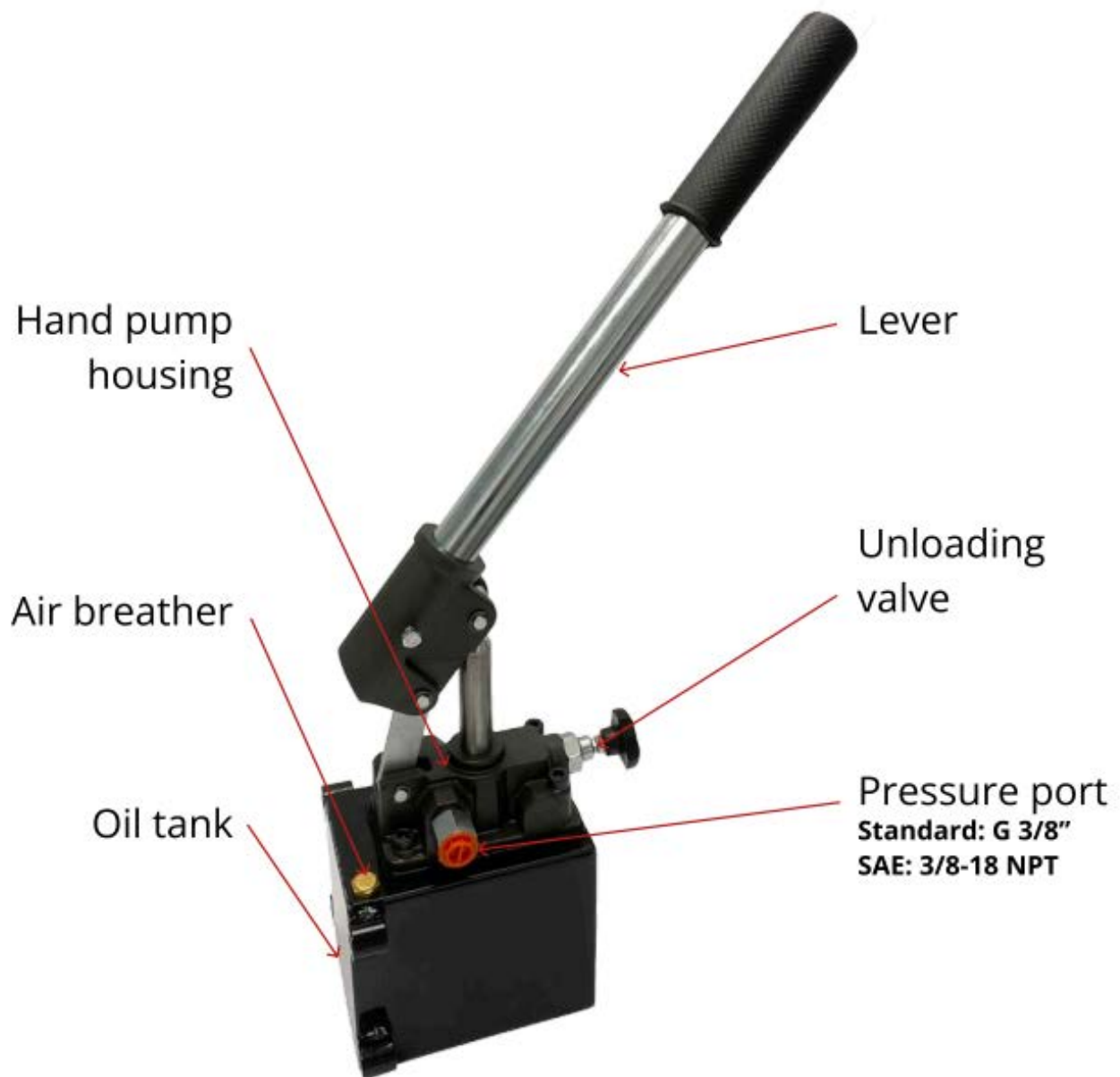
Photo 1. Main components of a single acting hand pump
